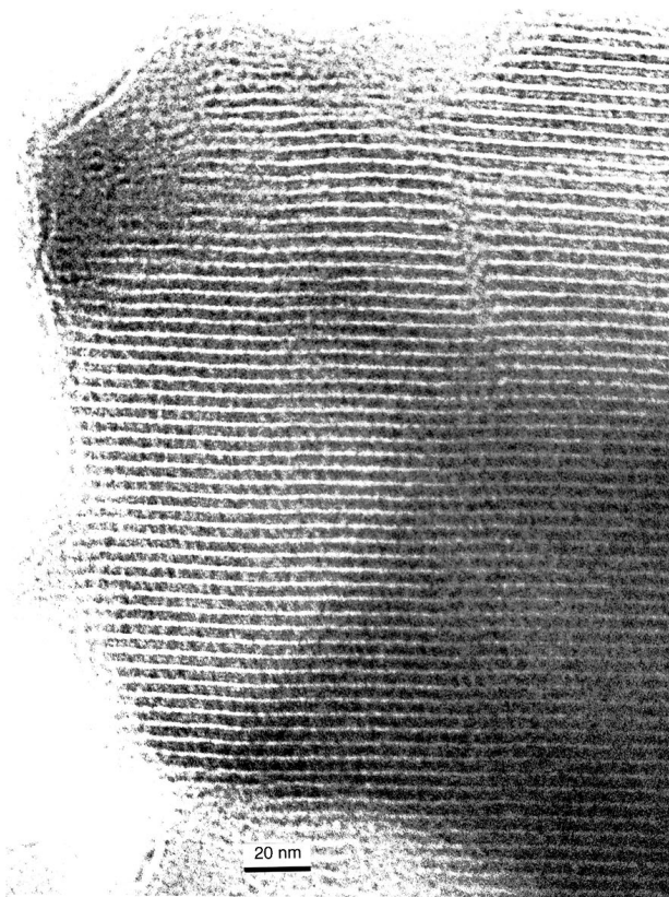
Fig. 3 HRTEM image of the Al-grafted AIMCM5 sample with a Si/Al ratio of 6.1.
